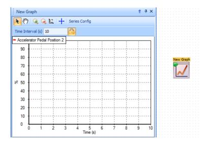
You may now configure the **New Graph** by referring to the **Graph Window Configuration** setting section described earlier in this manual. In addition you will need to connect the new **Graph** function block to the system using the **Drawing Pen** as described earlier in this document.
