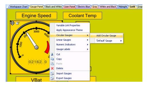
**Circular Scales, Circular Pointers**, and **Circular Ranges** can only be added to existing **Circular Gauges**, and similarly, **Linear Scales, Linear Pointers**, and **Linear Ranges** can only be added to existing **Linear Gauges**. An example showing how to add a **Circular Range** to the 'Default' Circular Gauge can be seen in the image below.
