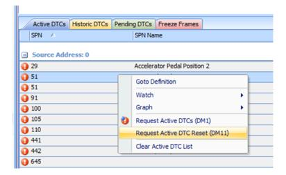
This will send the request out of the output port of the J1939 Diagnostic function block.
