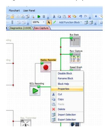
The **Properties** window will now open displaying all the settings for the recorder block.
