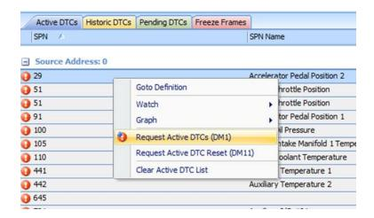
This will send a request out of the output port on the J1939 Diagnostic function block to the CAN bus.
