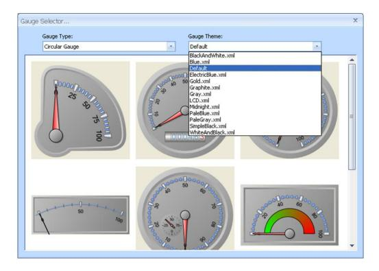
When you have found your desired gauge, double-click on it, and you will be prompted with a special mouse cursor signifying that a gauge control is about to be created. While this cursor is showing, simply drag and release a square area in the **Custom Panel** workspace to create a **Gauge Control** with the respective size.
